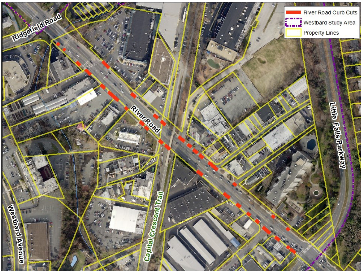
Figure B.3: River River Road Curb Cuts
